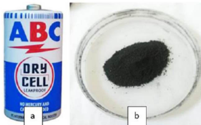
Fig. (1). a) A ZnC battery waste and b) graphite powder from the ZnC battery.
