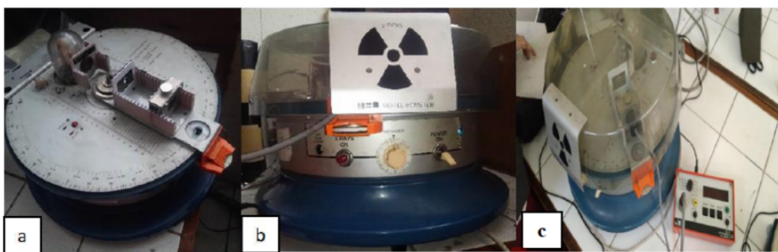
Fig. (2). The upper (a) and front (b) views of the X-ray generator. A GM counter is placed in front of the X-ray tube (c).
